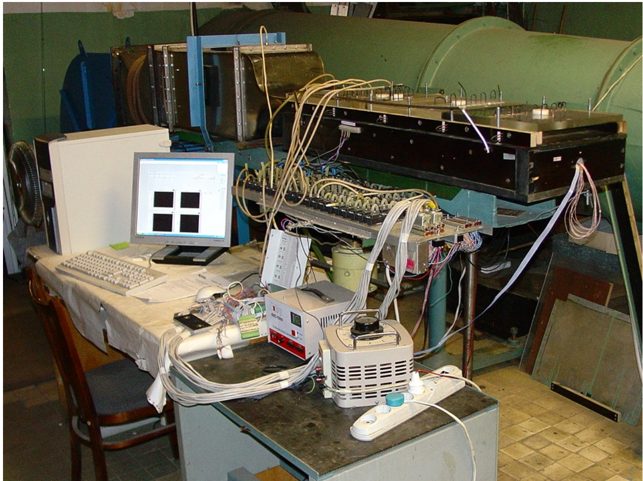
Fig. 9 – photo of the small aerodynamic test bench of the SRI of Mechanics of MGU
