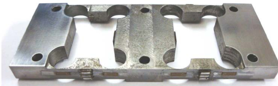
Fig. 11 Photo of the elastic element of the strain-gauge scale
